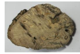
Fig.7. T.S. of borer infested kharsu oak log showing damage caused to Kharsu oak wood by larval galleries and chambers
