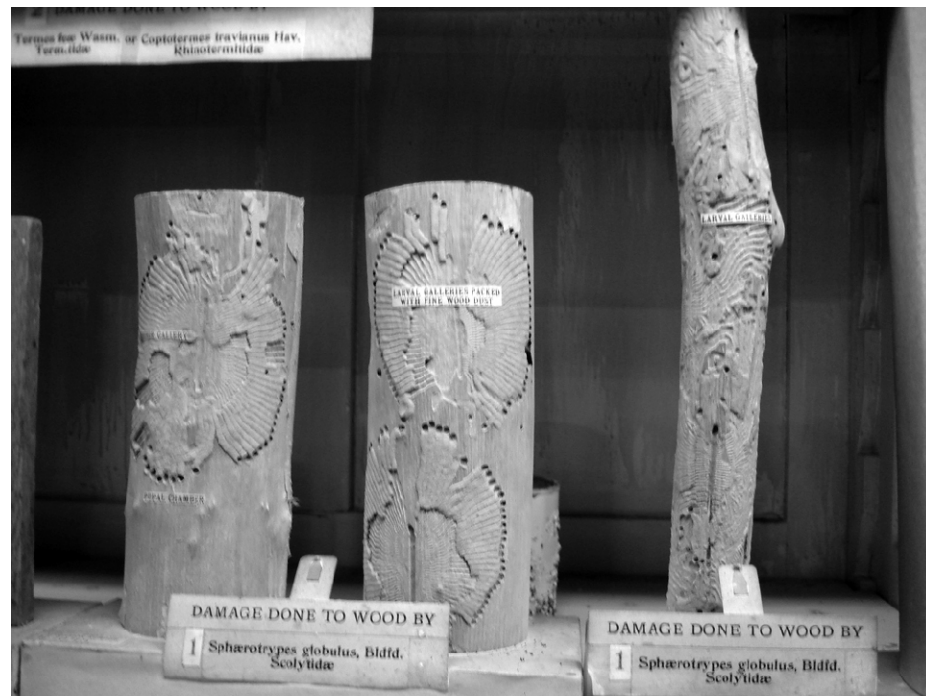
Damaged samples of wood of Lagerstroemia speciosa by Sphaerotypes globulus
