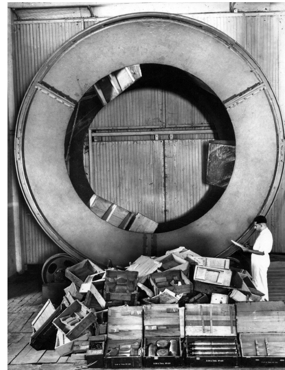
The drum box testing machine showing testing of ammunition boxes, Timber Testing Section, FRI Photo: M. Bakhshi, June 1941
