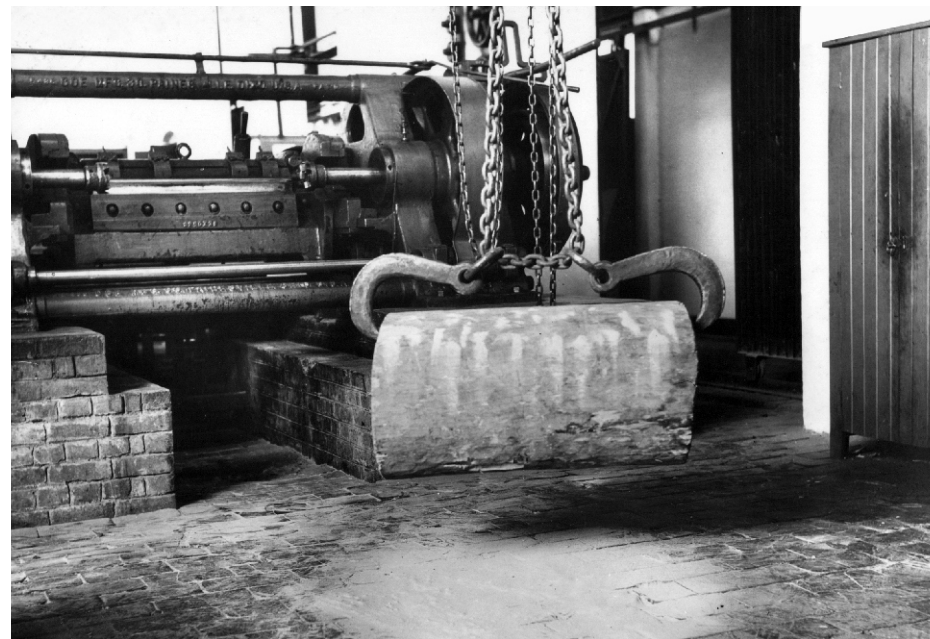
Borer attacked bolt of Terminalia belerica (from Baroda state), Wood Workshop Section, FRI Photo: M. Bakhshi, 01.07.1941
