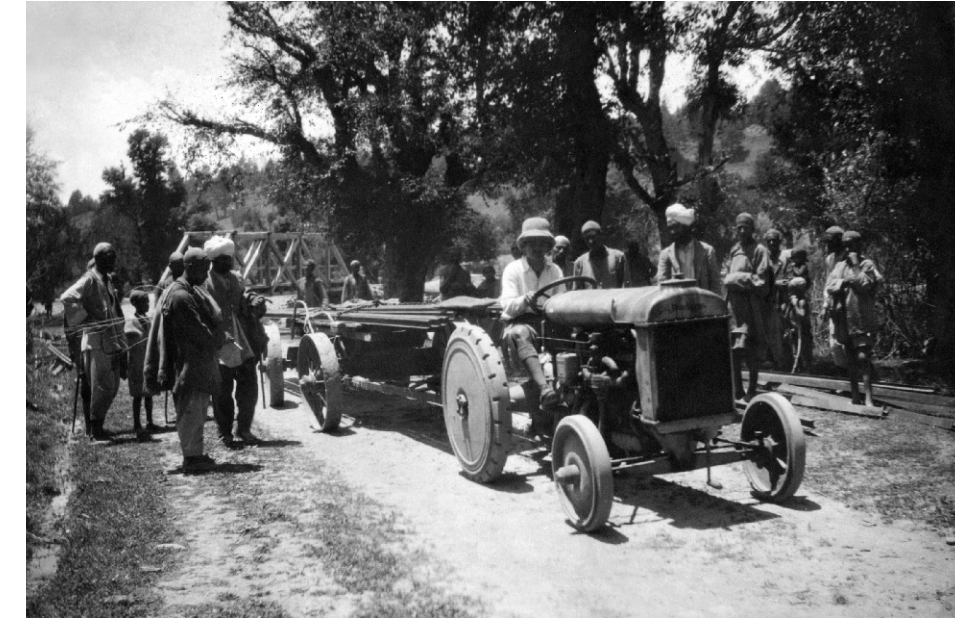
Fordson tractor and heavy iron 'Case Tractor' cart loaded with 20 lb. rails for tram line Photo: Bakewell, 1929
