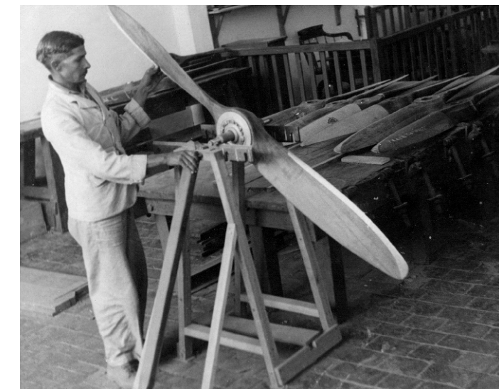
Balancing of a flight air screw on balancing machine at FRI Photo: British Ministry of Information, Delhi Office, FRI/WW (7)
