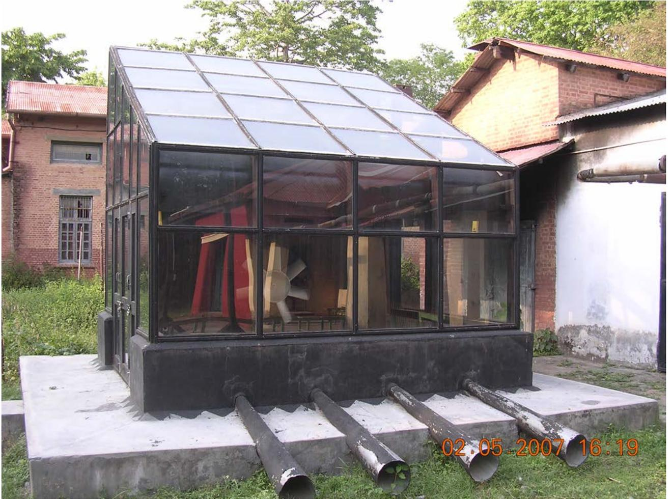
**Modified Solar Kiln for Timber Drying**
